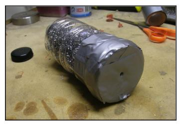
Wrap some duct tape around it to secure it altogether plus a few layers around the front. The idea is to fire a bullet through the tape to make the exit hole. The first shot will always be quieter but you can always just put another bit of fresh tape over the hole.
