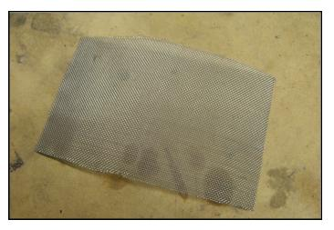
Cut a length of fine stainless or aluminium wire mesh
