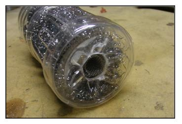
Fit the end cap back on with the tube of mesh just poking through so it can be supported.
