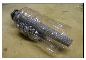
Start packing the scourer material around the tube. The fine mesh will stop strands of the scourer poking through into the path of the bullet which could lead to it being snagged and damaging the suppressor internals.
