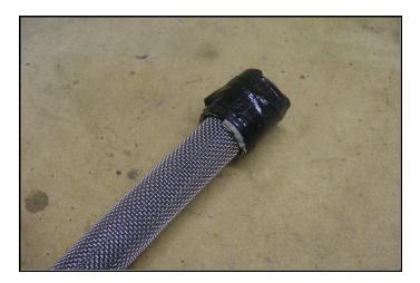
Wrap some cardboard and/or tape around the end of the mesh tube so it will fit snugly in the mouthpiece end of the bottle.
