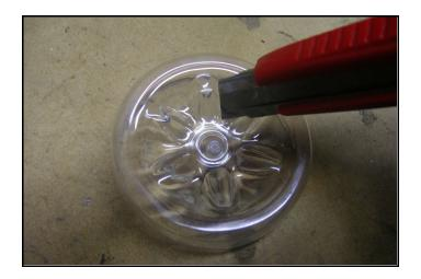
Either cut or drill a hold in the end of the bottle that you cut off earlier. The hole must be big enough to fit the tube of mesh through.
