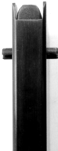
Photo 11: rear view of magazine with form block pinned in place
