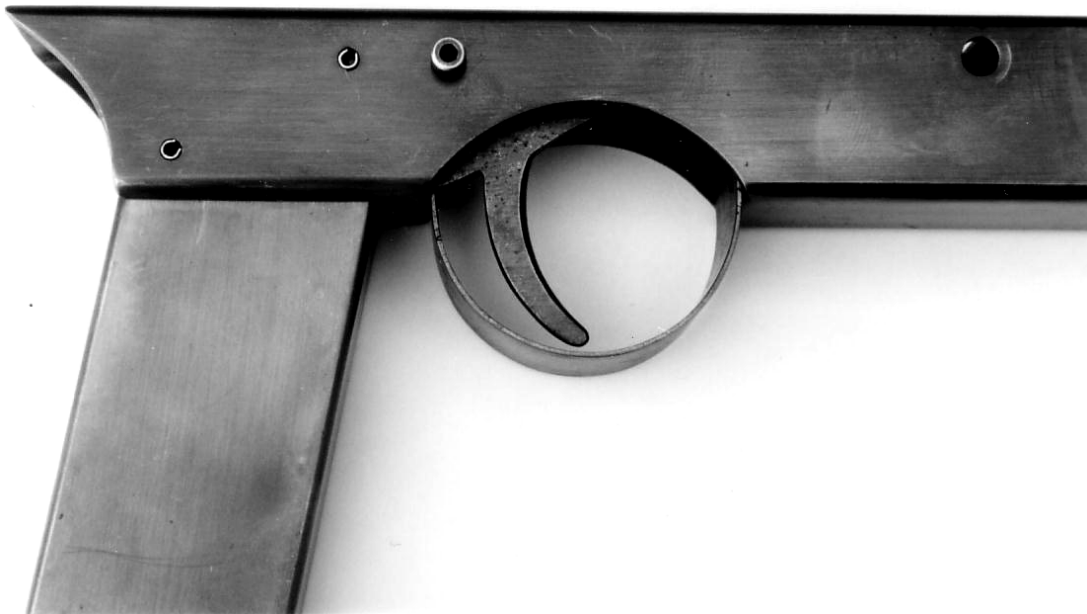
Photo 17: Trigger and guard fitted to receiver
