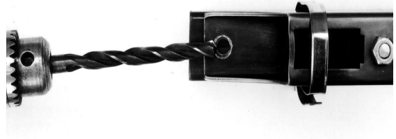
Photo 24: Drilling through the lower receiver bolt holes.
