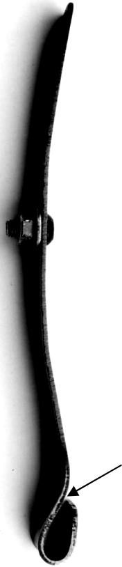
Photo 8: The magazine spring catch
